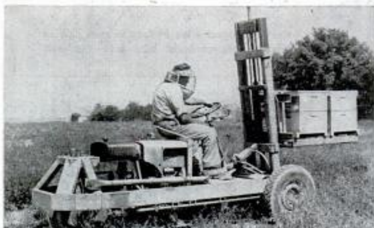
Another home-built machine is a hydraulic fork lift that will raise 1000 pounds to height of nine feet. Here it is used to move beehives to alfalfa field. Below, home-designed ditcher has two hydraulic controls to raise, lower and tip the blade
